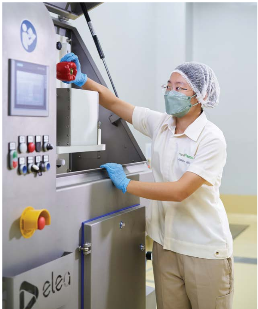
Non-Thermal Processing Room with pulsed electric field system.
