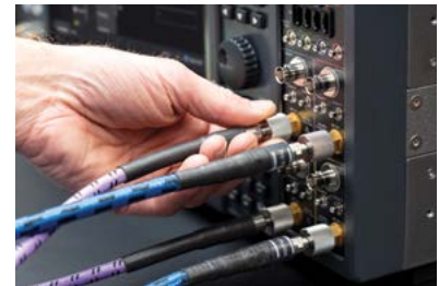
The vector signal generator provides four coherent channels in one instrument. Image: Keysight Technologies Inc.
