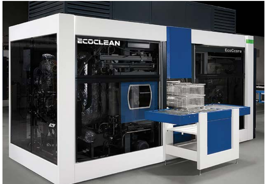
Modern solvent cleaning systems do more than just efficiently remove organic contamination, to achieve the required level of cleanliness. They also meet high environmental standards and significantly prolong the service life of solvents, thanks to integrated media treatment.
