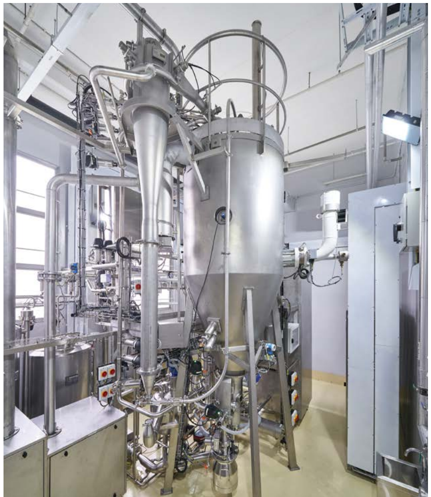
Multi-stage spray dryer with pressure nozzle atomiser.
